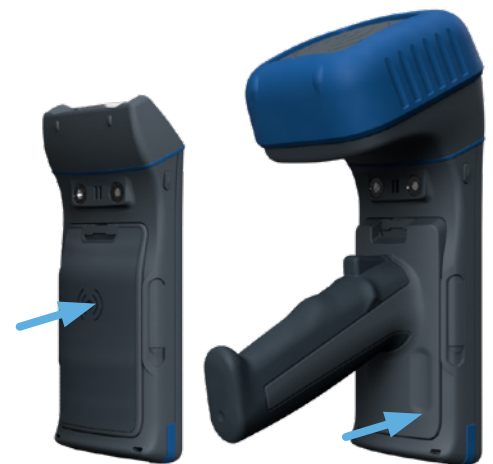
Position of NFC antenna in Brady HH83 and Brady HH85
